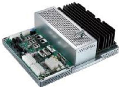
embedded platform, the DPX-E135 provides a complete PC platform with passive cooling. The system uses AMD's latest high performance dual and quad core SOC devices with "Discrete-level Graphics" from the integrated HD8000 series graphics core. A full feature set of I/O and COMs designed specifically for gaming devices is also included making the DPX-E135 an ideal integrated platform for many gaming,
